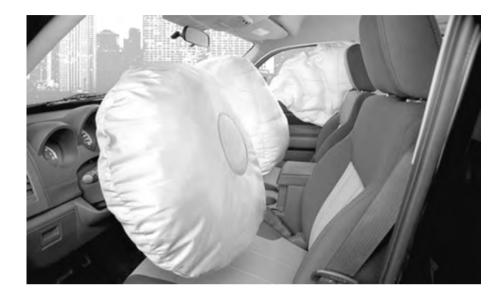
If a car is involved in a collision, the sodium azide decomposes.
